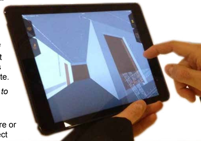
Above: Model of the New Østfold Hospital; Using Rendra O software, streaming 3D model to a tablet
