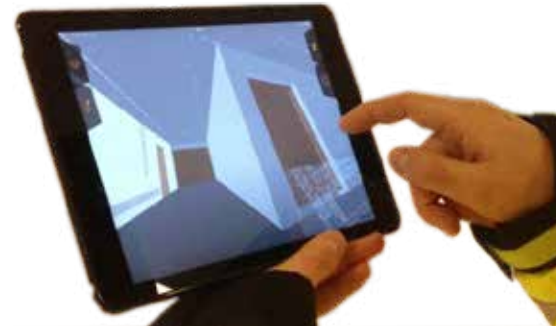
Top: Model (in Solibri), showing below-ground piling Below: Rendra O software allows the model to be streamed to personnel on-site on a tablet
